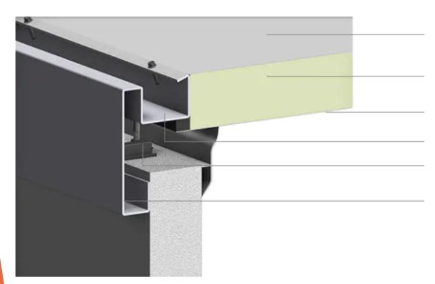
0.45mm colored steel sheet, color is optional, Aluminized zinc galvanized AZ50g/m2+PE baking finish15/5um
