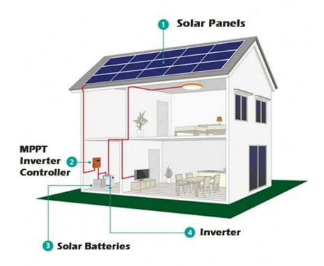
This solar kit is designed for a daily consumption of 20 kWh. Supplied with 20 solar panels (roof/ground mounting included), 250 w, 25-year warranty, 1 MPPT controller that can be connected to the generator to charge the batteries on cloudy days, 1 inverter, 8 x 250 AH batteries, 6 pairs of connectors and 100 meters of cable.
